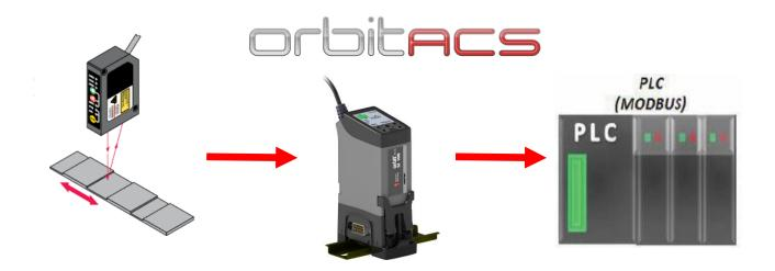
Easily connect Orbit® LT to PLC via SI 100, SI 200, or SI 400 interface module.
