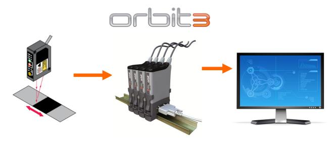
Network Orbit<sup>®</sup> LT with other gauging probes or sensors via the Orbit<sup>®</sup> 3 network.
