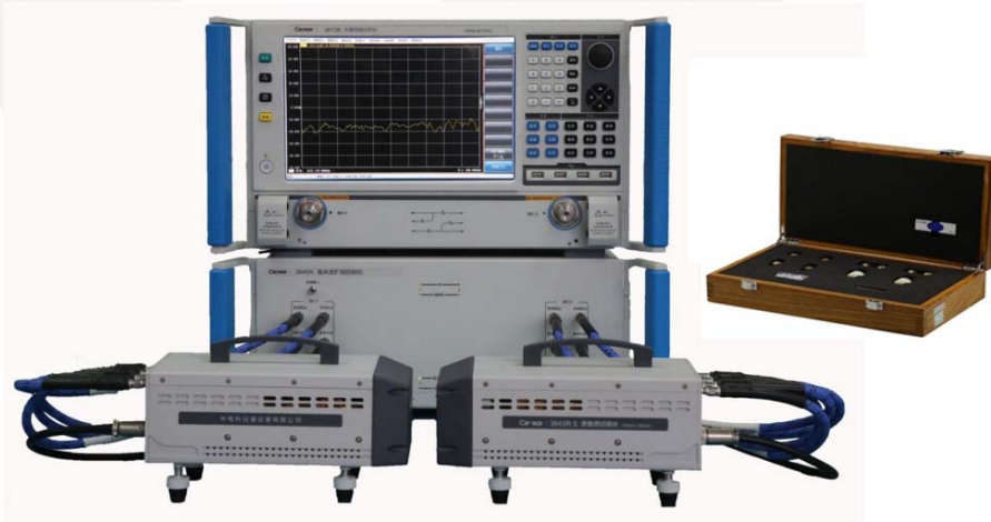
Fig. 4 Mm-wave and THz VNA System (Type-II: based on 2 ports VNA and controller)
