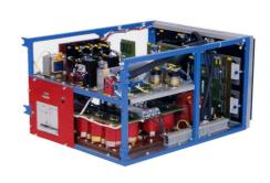
12kV PD test set for frequency converters of traction drives
