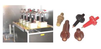
75kV PD- test set for automated PD-tests of cast resin bushings with a high voltage switching device in a screened test room
