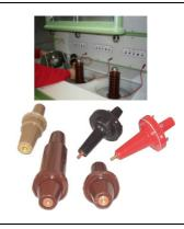
100kV PD test set for automated tests of surge arresters in two test chambers
