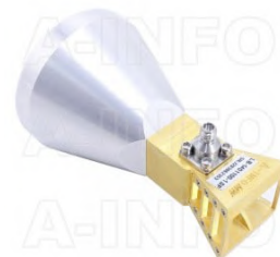
LB-1401100-1.0F Broadband Horn Antenna 14-110GHz 13dB Gain 1.0mm Female
