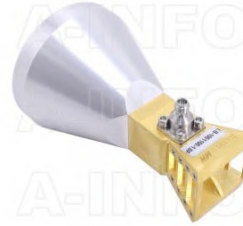
LB-1001100-1.0F Broadband Horn Antenna 10-110GHz 13dB Gain 1.0mm Female
