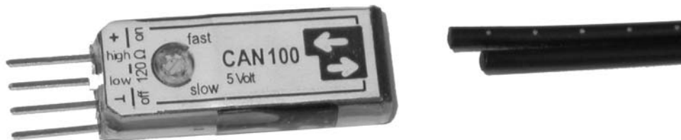
Figure 3 CAN 100 connection with the optical fibre
