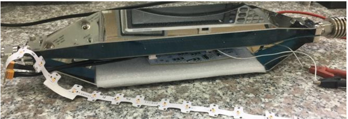
Picture 3: DUT inserted into the TBTC0 TEM cell
