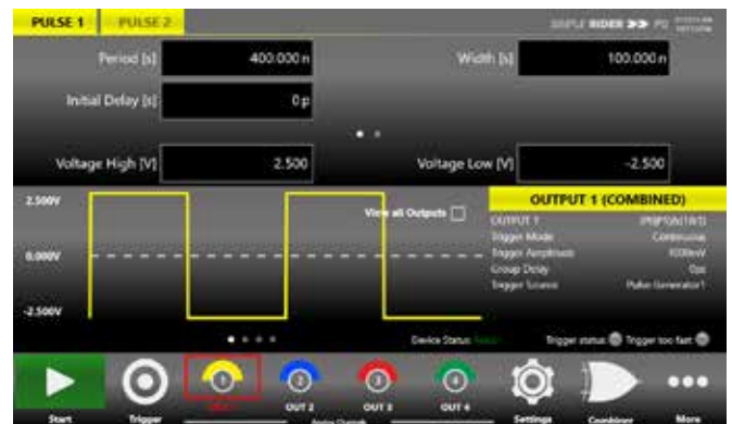
Figure 2 Simple Rider UI, generation of two narrow pulses (5 ns) with 7.5 ns of Delay(s) one from the other.
